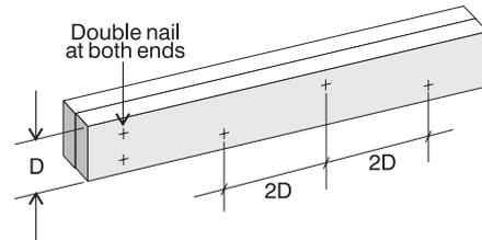
Figure 5 - Multiple beams
